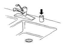
The drain air gap is usually located on top of the sink or countertop near the dishwasher. To order a drain air gap call 1-800-366-7278 and ask for Part Number 300096.
